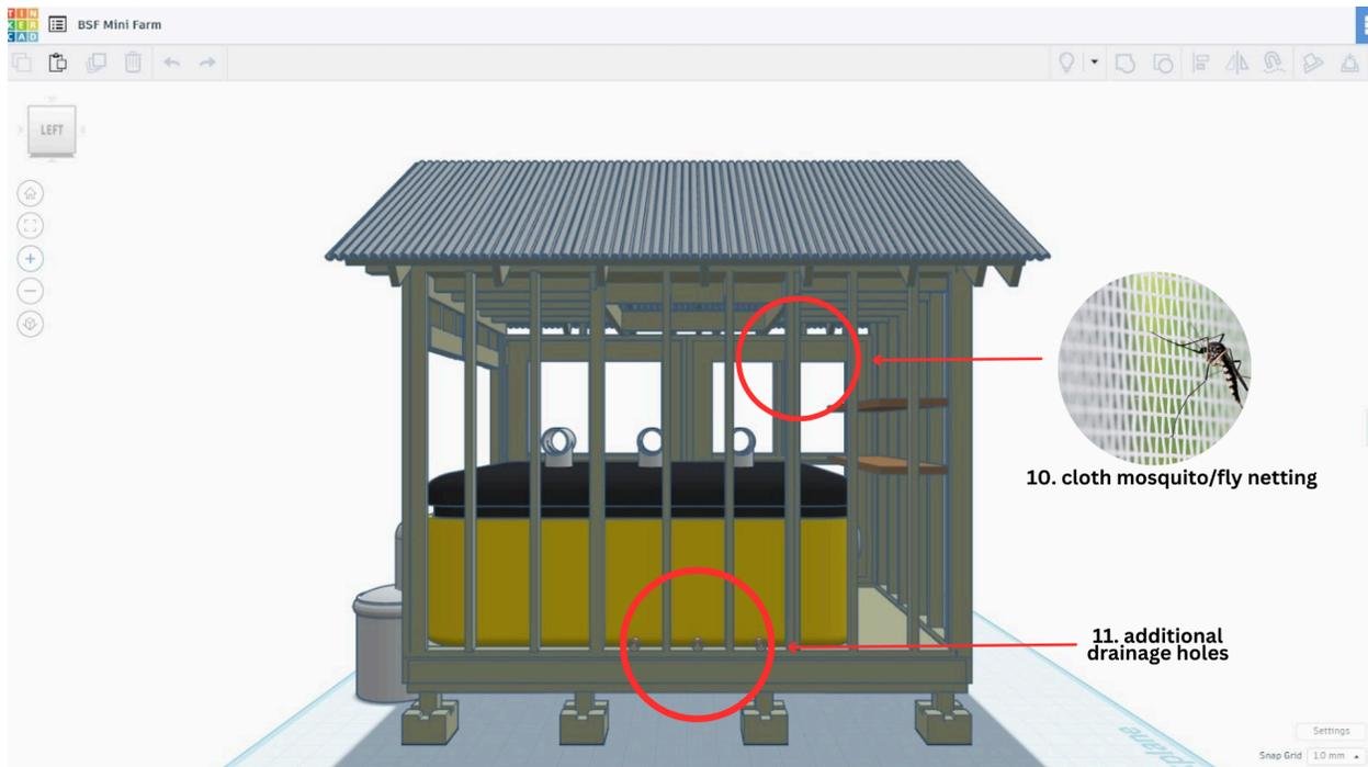
Figure B5. Labelled rear section view of the composting system.
