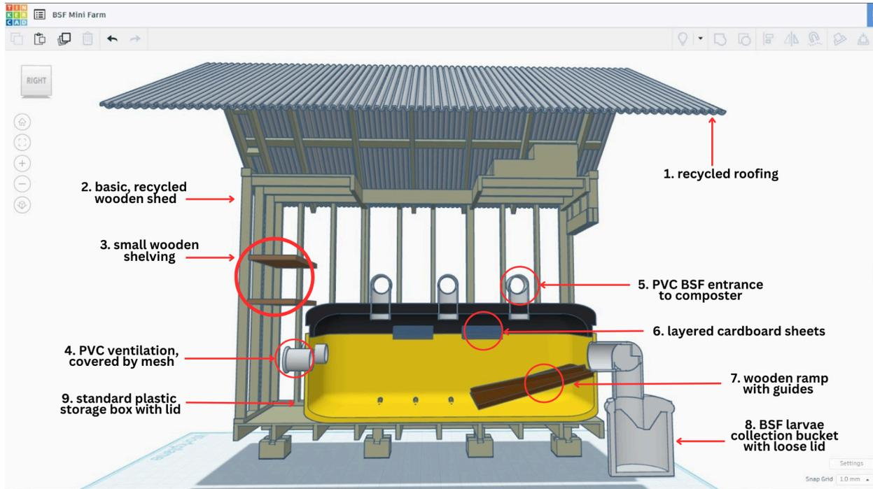
Figure B4. Labelled front section view of the composting system.
